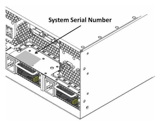
Figure 3-4 System Serial Number Label
